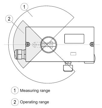
Fig. 1 – Measuring and operating ranges
